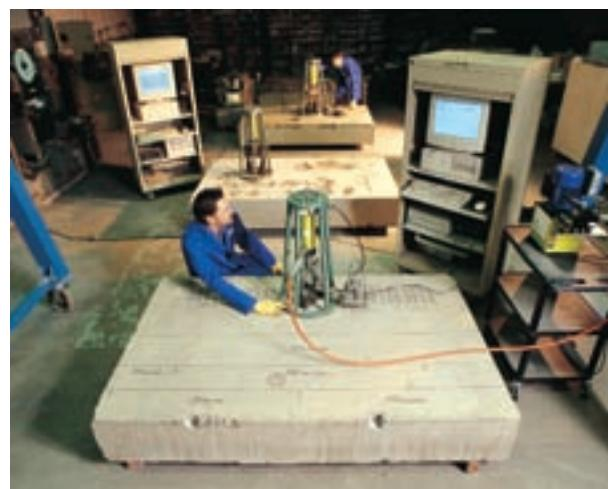
– checking the percussion characteristics of the fixings throughout its life span.
